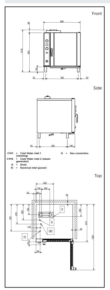
Electric Supply voltage: 260819 (EFCG11CSAS) 220-230 V/1 ph/50 Hz **Auxiliary**: 0.35 kW 0.35 kW Electrical power max.: Gas Gas Power: 18.5 kW Capacity: Trays type: 10 - 1/1 Gastronorm
